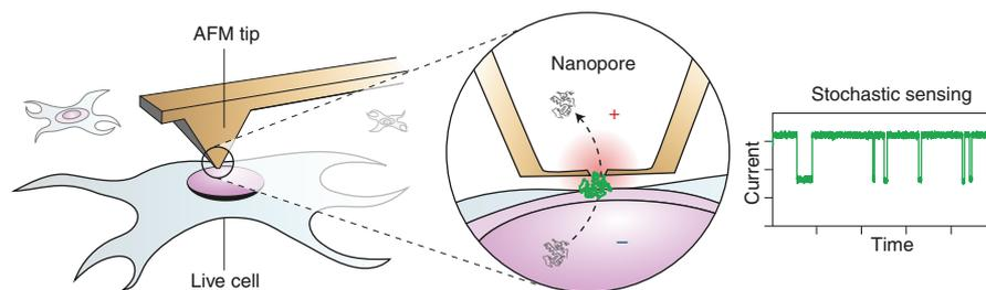
**Fig. 1 | Schematic of the AFM/nanopore tip in operation.** A nanopore probe made at the centre of a flattened AFM tip enables in situ stochastic sensing of secreted biomolecules when used to scan the surface of live cells.
